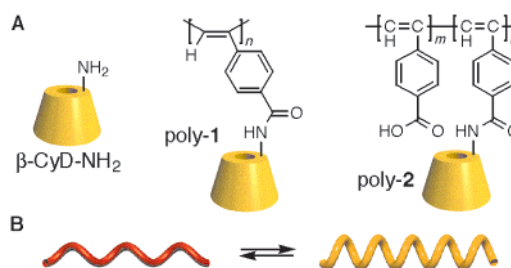
Figure 1. Structures of \beta -CyD-NH 2 , poly-1, and poly-2 (A) and schematic illustration of interconvertible right- (red) and left-handed (yellow) helices of poly-1 (B).
